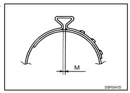
9. After installing housing and shaft, rotate boot to check whether or not the actual position is correct. If boot position is not correct, remove old boot bands then reposition the boot and secure with new boot bands.
