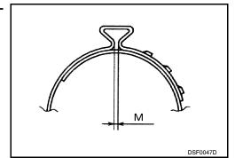
9. After installing housing and shaft, rotate boot to check whether or not the actual position is correct. If boot position is not correct, remove old boot bands then reposition the boot and secure with new boot bands.
