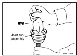
Cover serrated part of shaft with tape. Install new boot and boot band onto shaft. Be careful not to damage boot.
