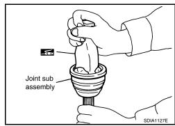
Cover serrated part of shaft with tape. Install new boot band and boot to shaft. Be careful not to damage boot. CAUTION:
