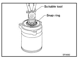
Press support bearing assembly off slide joint assembly using a suitable tool.
