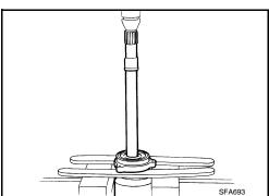
4. Separate support bearing from retaining bracket using a suitable tool.
