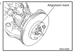
Remove wheel sensor from steering knuckle. Refer to <u>BRC-202, "Removal and Installation"</u>.
