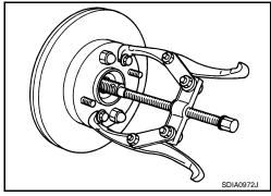
10. Remove wheel hub and bearing assembly bolts using power tool.
