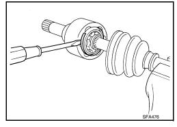
6. Put matching marks on spider assembly and shaft.
