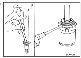
2. Remove snap ring using a suitable tool.
