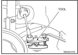
8. Remove transverse link to steering knuckle pinch bolt and nut using power tool.
